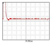
Changing the effective output impedance only had very little effect on the current. It is the reason that current-amplifiers (instead of voltage amplifiers), like the Bakoon, which by nature have an extremely high effective output impedance, do work well with magneplanar headphones.
