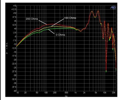
Fortunately, the HD800 has a very high impedance to start with, but, as Jan mentioned, many of todays portable headphones have very low impedances, and that means that they'll be even more sensitive to amplifier output impedance. For example, here's the Sennheiser PX100 impedance curve.
