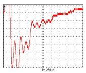
On the other hand, when increasing the output impedance the oscillations get smaller and smaller and are completely gone at +88 Ohm.
