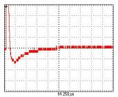
The HD-800 has a relatively high coil-resistance of 300 Ohm. Thus there is enough resistance available for proper damping. However, over the years there has been a clear tendency towards headphones with much lower impedance values. The reason is simple. They go louder with lower signal voltages—the output voltages of modern portable players is very limited...and for many the louder the better.
