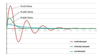
3. When the value of R is increased to a value where in the formula above w=0 the signal no longer oscillates. After an initial bump the signal continously decays and goes to zero relatively quickly. This situation is called critical damping and is shown by the green line. R = 200 Ohm.
