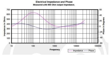
Again, look at the impedance plot of the HD800. With a high output impedance amp, the headphones will get a little more gain as the impedance goes up. Therefore, you can think of the impedance curve as an EQ curve with high impedance amplifiers. The higher the amp output impedance, the more the headphones will be EQ'd toward the shape of the impedance curve. In the case of the HD800, the higher the output impedance of the amp, the more you'll get a midbass boost centered at 100Hz.
