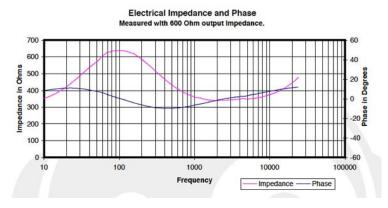
In the above plot, you can see that the Sennheiser HD800 has a peak impedance of about 650 Ohms at 100Hz, and a low impedance of about 350 Ohms at 3kHz. I'm going to try to keep the math easy here for illustrative purposes, so let's say it's 600 Ohms at 100Hz and 300 Ohms at 3kHz.
