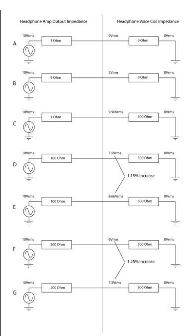
Here's a series of very simple circuits. The left side is the headphone amp and the resistor models the output impedance of the amp, and on the right is the headphone with the resistor modeling the headphone impedance. To the far left of each circuit is a signal generator putting out a 10Vrms signal. The 10Vrms signal has to go through both resistors to get to ground on the other side.
