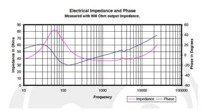
It's roughly 10% of the impedance of the HD800, and therefore you're likely to see changes in the frequency response curve like the HD800 with the differences in output impedance of only 0,10, and 20 Ohms... and that's near the normal variation of portable devices. Fortunately the PX100 could probably use a little more bass.
